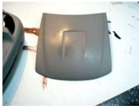
We had to build up the hood with putty to reform the scoop to match the GT before primer and paint.
