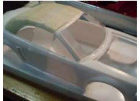
The 96-windshield frame was installed on the 99 body using the top and glass for location.
