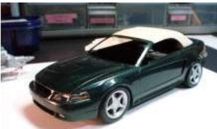
After a couple more coats of paint and clear, it was allowed to dry a couple of days then wet sanded and polished. The next step was the final test fit before assembly.
