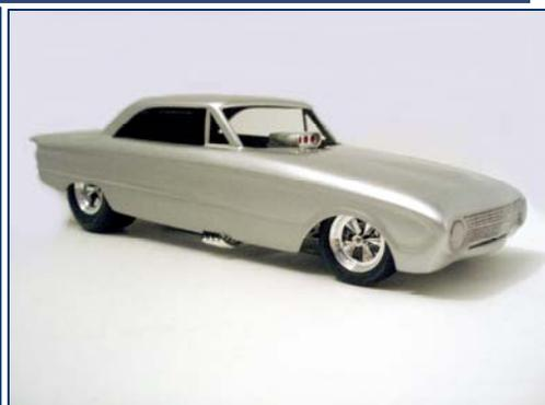
Step 11 - The windows were cut from a sheet of clear acetate and mounted into the body. The body was then fitted to the chassis and final details added.
