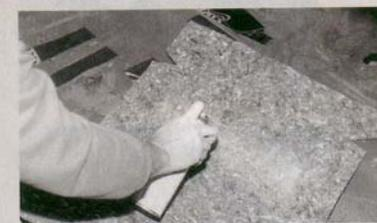
These sound-deadening pads not only keep out noise, they keep out heat and cold as well. Spray the trim adhesive, included in the kit, in liberal amounts on the back. Allow to tack off for five minutes. Then, lay it down.
