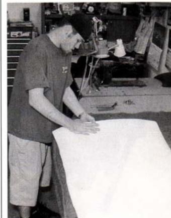
We see a lot of interiors with loose-fitting vinyl. There is a way around this. Mike Ambrose Custom Interiors in North Hills, California, lays down 1/2-inch layer of foam over the gauze material. This fattens up the seat, and makes it more comfortable to boot.
