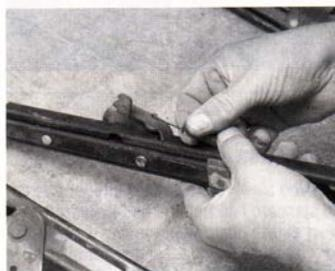
Whenever you are reupholstering seats, clean and lubricate the seat tracks for smooth, reliable operation.
