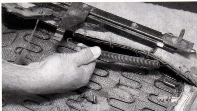
One of the most important seat tricks is protecting yourself. Before removing seat tracks, always carefully remove the helper spring, which will reduce the risk of injury from a runaway seat track.
