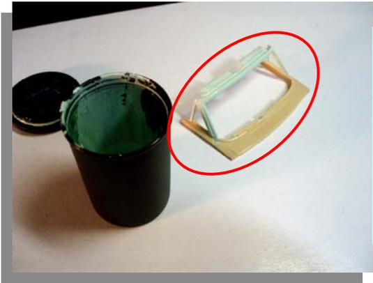
Because the finish on the body was so good, I decided not to paint the body but mix some paint to match the body color and paint the new resin windshield frame. I then polished and buffed the body before I glued the windshield frame the body.
