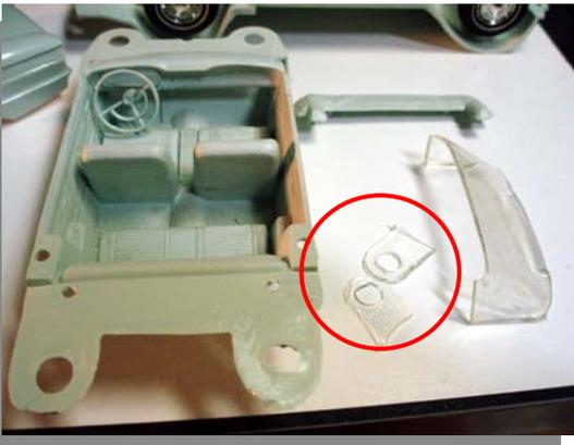
As I disassembled the car I noticed that the windshield tabs were broken and would have to be repaired and polished. The axles and mounting screws were very clean and needed little or no clean up.
